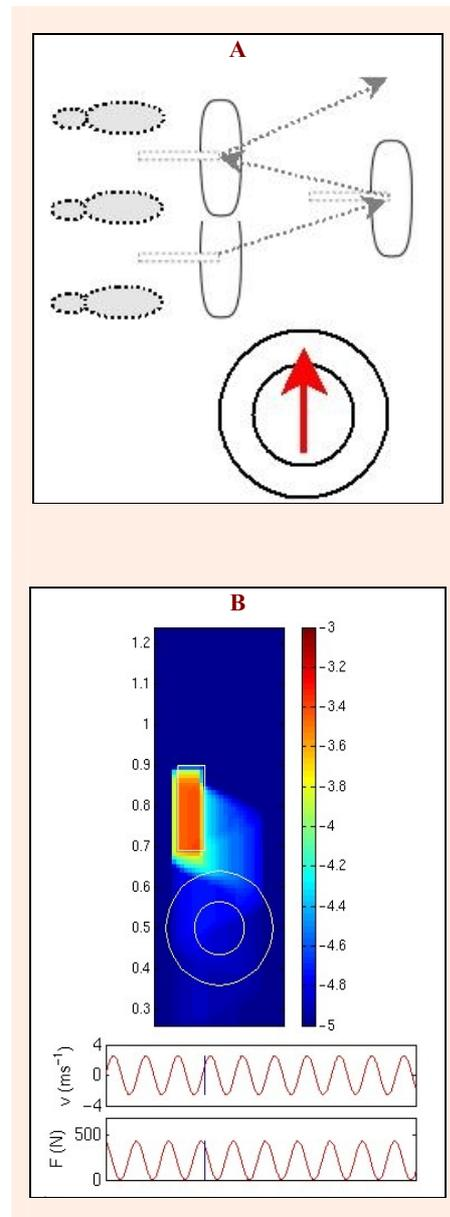
**Figure 2.** Sweeping the same piece of ice more than once. **A** illustrates the position of the curler with respect to the stone in conventional sweeping. **B** is a thermal animation of the heat generated from conventional sweeping [thermal movie reproduced with kind permission from Marmo et al (2006b), available from URL: <http://www.jssm.org/vol8/n4/1/curling.htm>].
